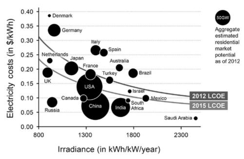
Note: LCOE based on 6% weighted average cost of capital, 0.7%/year module degradation, 1% capex as O&M annually. \$2.65/W capex assumed for 2012, \$2/W for 2015.
